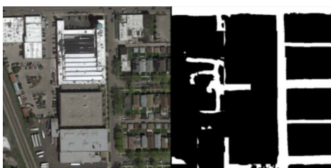
Figure 6: The parking on the left of the image is badly delimited and contains weird looking road predictions.
